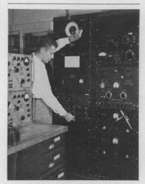
STRAIGHT FROM WASHING-TON comes the radio signal of WWV, Bureau of Standards. In this picture Richard Carpenter is checking the laboratory clock against the call.
